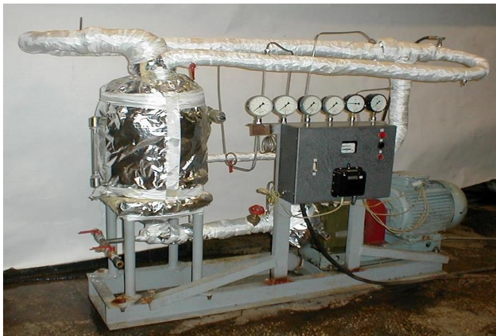
Рис. 5. Natural view of cavitation installation (version 1)
